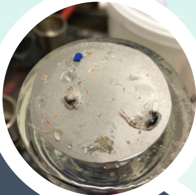
TOP RIGHT: Material collected in a manta net from the Mediterranean Sea (2019). MIDDLE and BOTTOM RIGHT: Material collect in the manta net is captured on a stainless-steel filter (10-µm mesh size), where larger plastic particles can be seen alongside small biota. (Photos: Julia Farkas, SINTEF Ocean)
